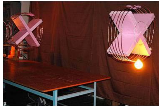
Fig.3 Evanescent wave coupling
